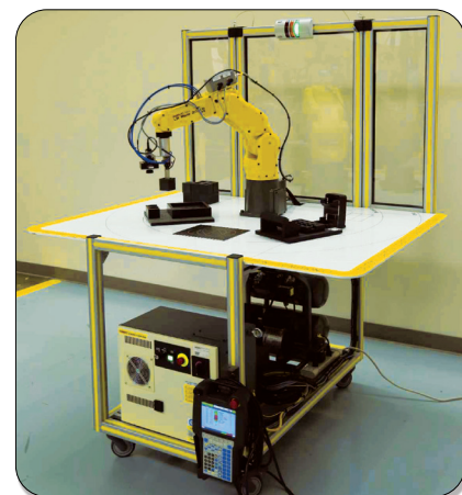
FANUC LR Mate 200iD/4S Fencelless CERT Cart
