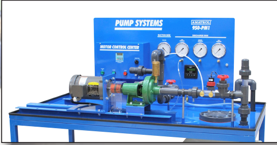
Centrifugal Pump (green) on the 950-PM1
