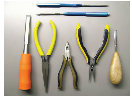
Figure 16: Remove supports using the proper tools such as a chisel, magnetic handle pick set, pliers, and needle nose pliers.
