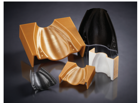
Figure 1: The high heat resistance and low CTE of ULTEM 1010 make it ideal for tooling applications such as composite layup tooling.
